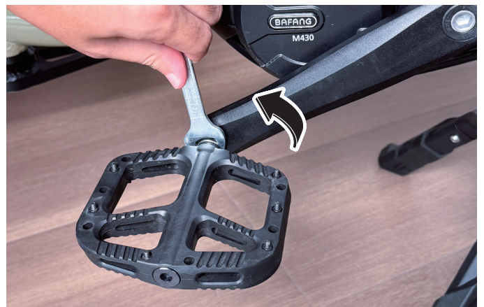
L Left pedal installation completed
